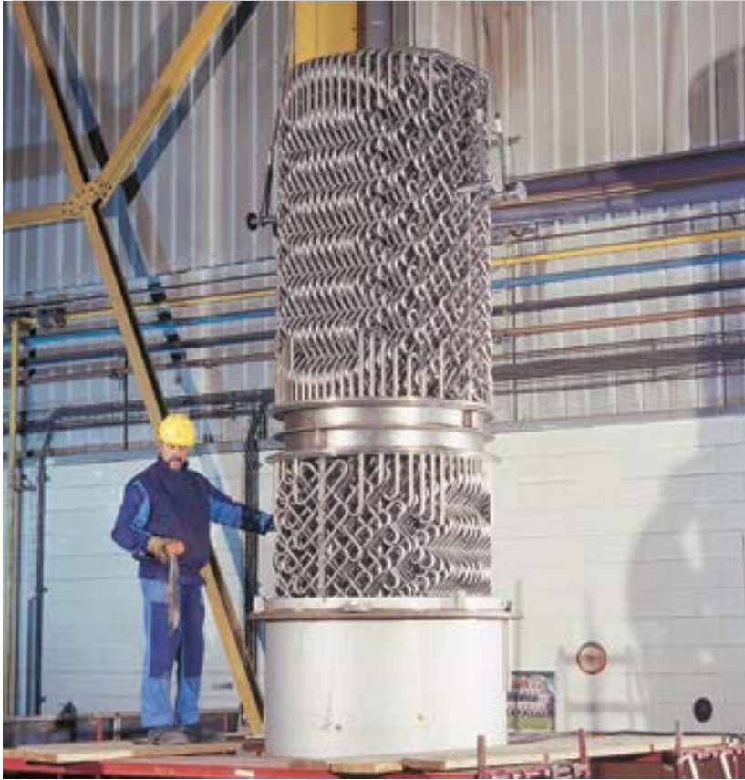
SMR™ static mixer reactor (Sulzer Chemtech)
