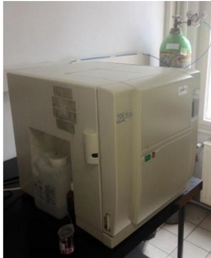
Fig. 3. Total Organic Carbon Analyzer TOC – TOC-VCPN Total Organic Carbon Analyzer, Shimadzu
